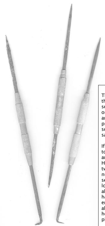
These are three machinist's scribes that I have used as solder picks for soldering for some time. Notice that on two of them, one end is straight and the other is bent. That was probably true for the third one at some point in time until I filed or sanded it away.
